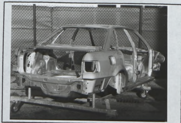
A10) Coque vue de 3/4 arrière, sans portes, capots, etc. Bodywork seen from 3/4 rear without doors, lids, etc.
