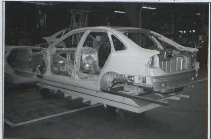
A10) Coque vue de 3/4 arrière, sans portes, capots, etc. Bodyshell seen from 3/4 rear without doors, lids, etc.
