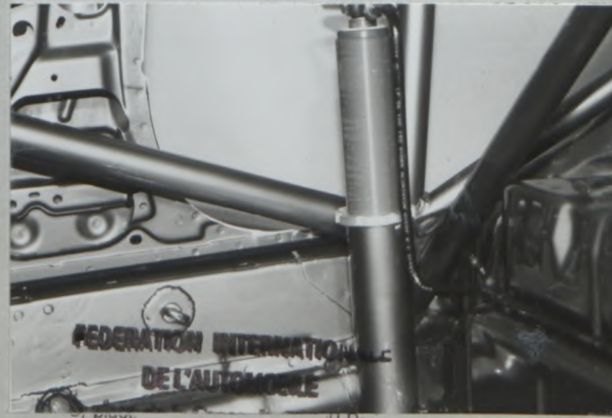
PHOTO No. 6 (MAIN ROLL BARS TO FLOOR)
