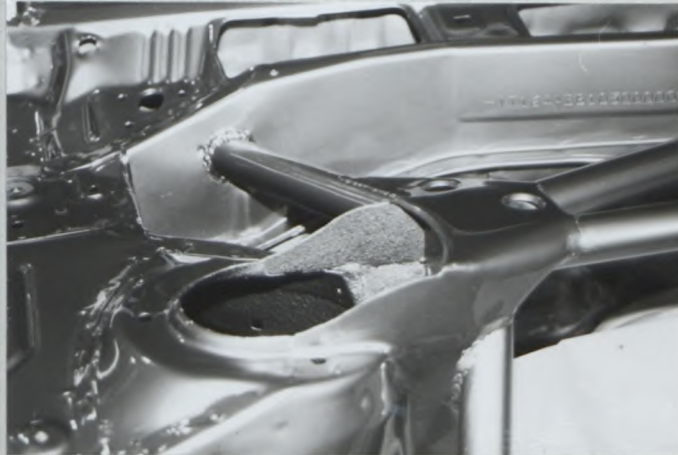
PHOTO No. 2 (FRONT SUPPORT BARS TO FRONT STRUT TOWER)
