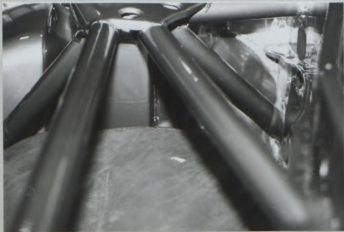
PHOTO No. 3 (FRONT SUPPORT BARS TO FRONT STRUT TOWER)
